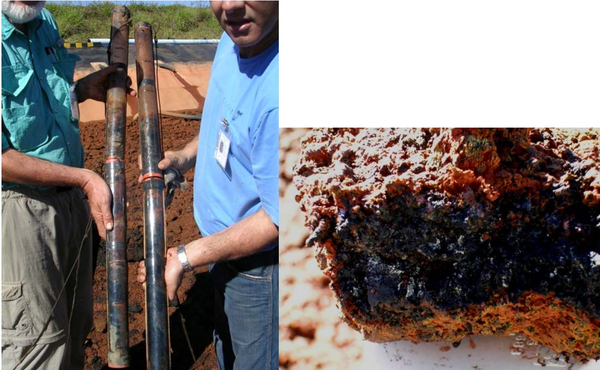
Figure 7. Pictures of the cores after 10 months in the full-scale ZVI cell and a clod from the surface of the reactor.
