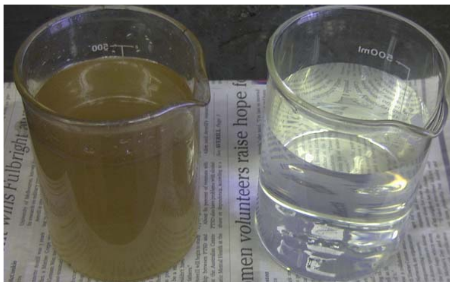
Figure 2. SPW before (left) and after treatment (right) by PA/O 3 /10 cy/SF and PA/O 3 /20 cy/SF (flowrate = 5 L/min).
