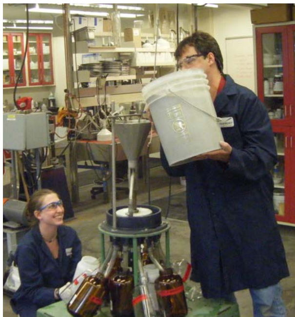
Figure 1. Using the slurry splitter to prepare the aging aliquots.
