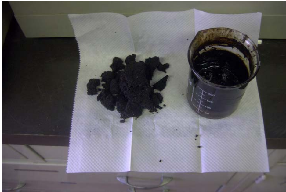
Figure 1A. Raw oil sand samples (12 % bitumen by wt.) of Asphalt Ridge, Utah (left) and collected bitumen (right).
