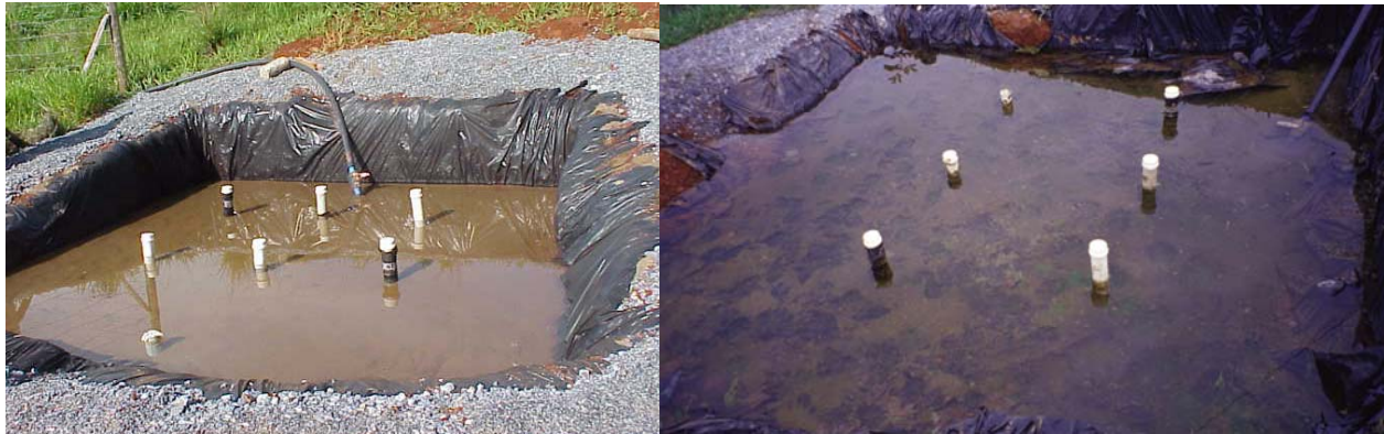
Figure 3. The top of the ZVI pilot cell in the beginning (left) and after 12 months (right).
