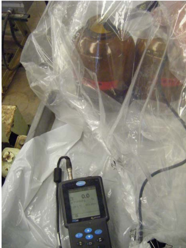
Figure 3. The glove bag and the oxygen meter showing that the slurry bottle was purged to anoxic conditions.
