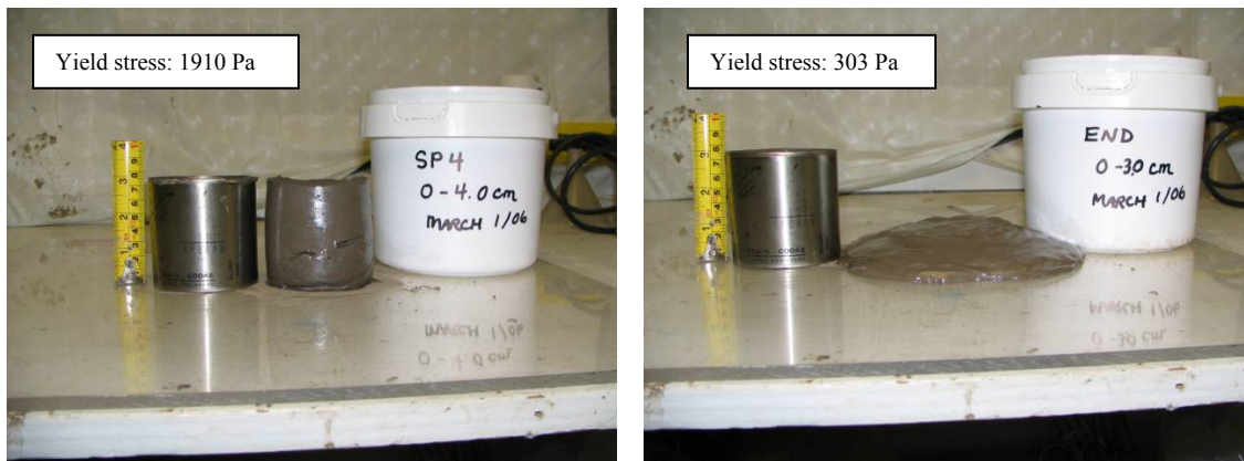
Figure 9. Yield stresses measured with VT-550 viscometer compared with cylinder slump tests.
