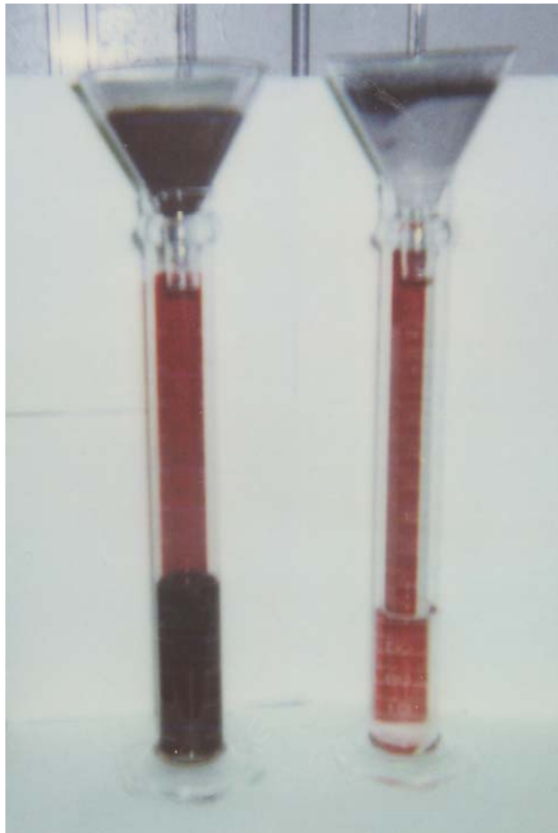
Figure 9. Humate Sand Filtration
