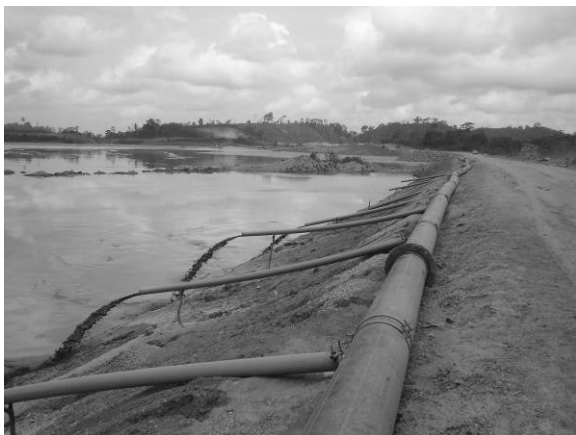
Figure 3. Deposition of tailings at the Wassa tailings disposal facility
