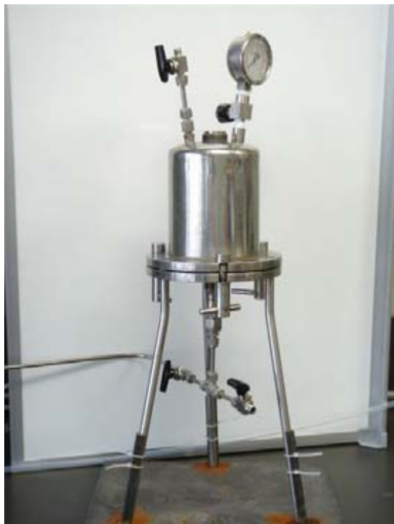
Figure 1. The feature of pressure reactor. There is a gas vent and a pressure gauge at the top, inlet and outlet at the bottom, and a magnetically coupled stirrer.
