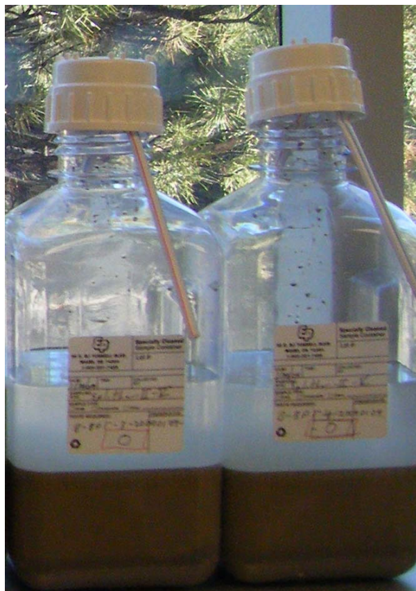
Figure 2. Oxic aging samples shortly after being split and rolled.
