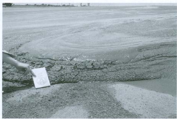
Figure 5. Thickened tailings (paste) being deposited (Lord et al., 2002).
